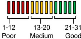
For good performance, signal level on 2G should be at least 13. On 3G products it should be no less than 10.
