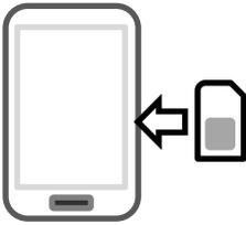
Please ensure the SIM card is a 3G/4G compatible Nano SIM card. The SIM may also be 2G capable as well, as long as both the SIM and the network also support 3G/4G. Do not use a SIM card for a tablet, as these only support data, and do not support voice and SMS. You simply require a mobile phone type SIM card.
