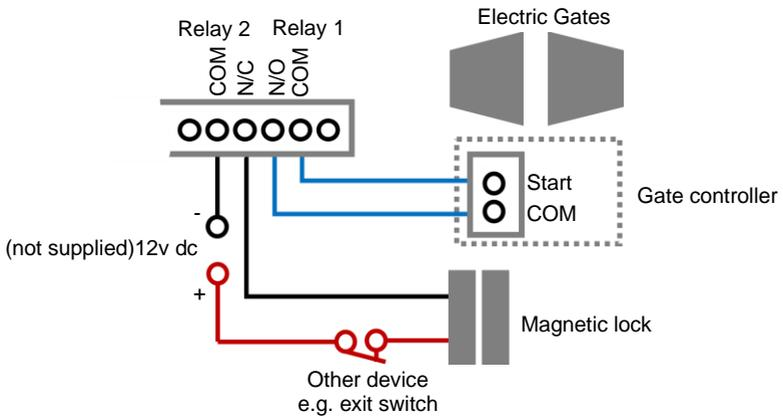
This example shows relay 1 connected to a gate motor controller for vehicle gates, and output 2 connected to a magnetic lock for a door or pedestrian gate.
